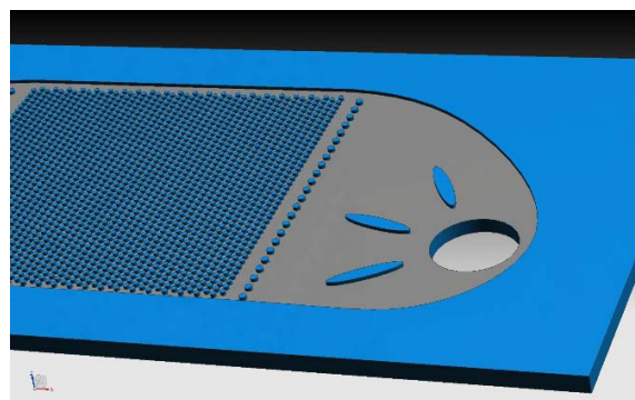
Fig. 11. Bonded regions (blue) for ideal bonding scenario
