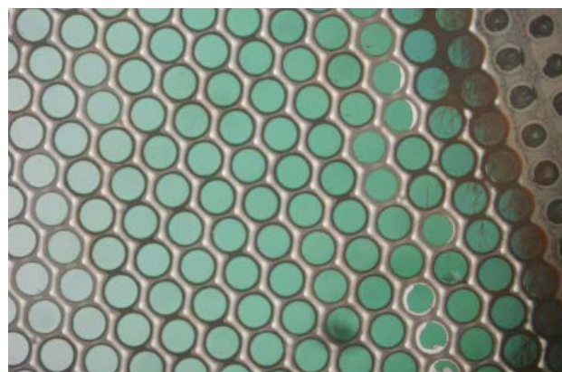
Fig. 9. 150 \mu\text{m} diameter pin-fin heads after fracture (still covered by glass)
